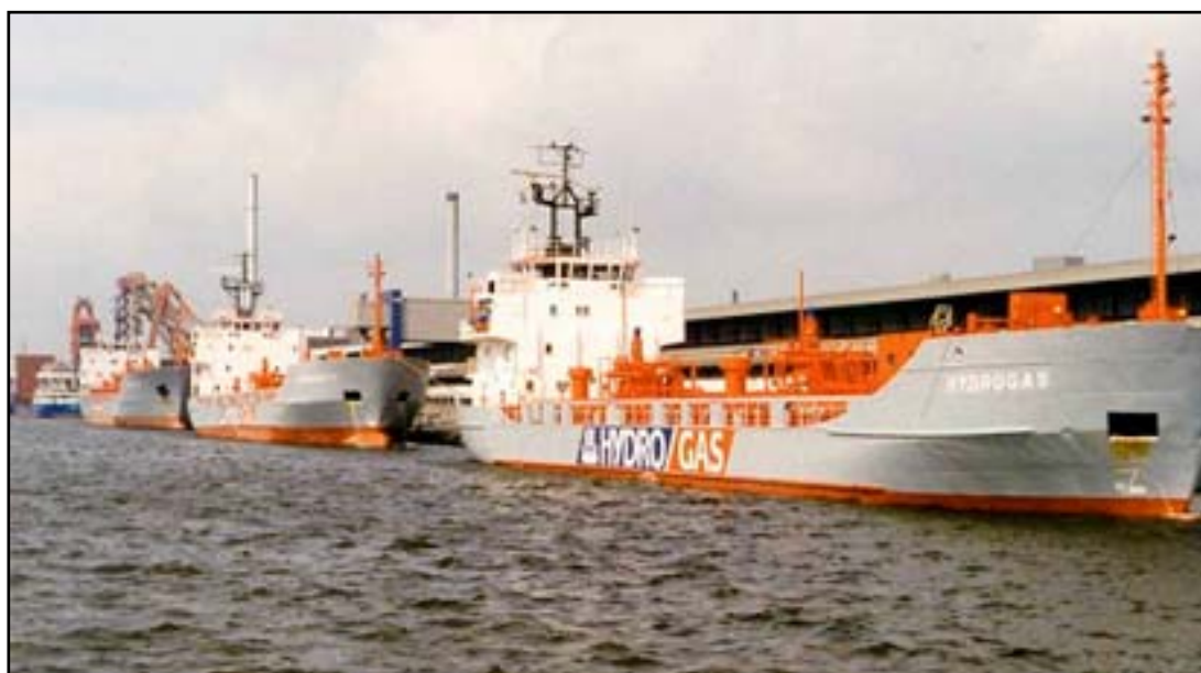
Fig. 8: Three of the CO 2 -ships owned by Hydro Gases and Chemical shown in port. Each has two CO 2 -tanks with total capacity between 900-1200 tCO 2 for each ship. Maximum speed is 12 knot.
