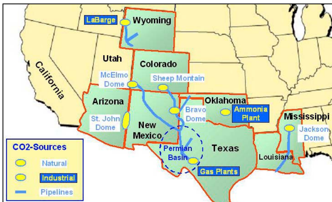
Fig. 1: Map showing CO 2 sources, transportation pipelines and extent of CO 2 -EOR in the South and South-West United States. The Permian Basin is the worlds largest CO 2 -flood region. The first flood was opened in 1972, but there are now over 50 active projects producing more than 145,000 bpd. The 1,500 km pipeline infrastructure from McElmo, Sheep Mountain and Bravo Dome delivers more than 23 mtCO 2 /yr. In year 2000 with oil at $18 /bbl the average price of delivered CO 2 was $12 /tCO 2 (Source: KMCO 2 and Jarrell et al., 2002).
