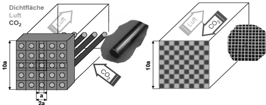
Figure 23. Possible structures for membrane reactor in the oxycoal-AC cycle (Renz et al., 2005).
