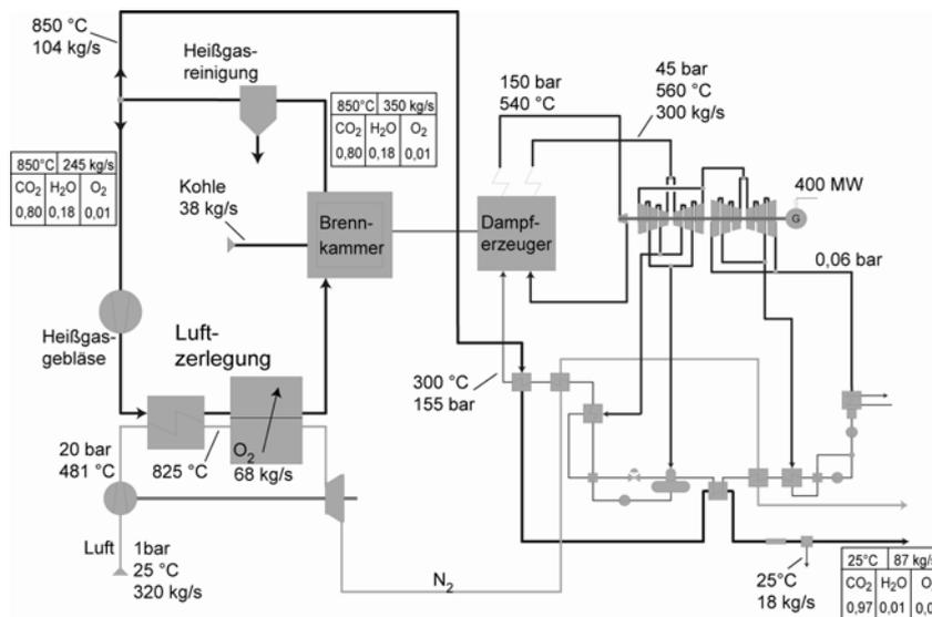
Figure 16. The oxycoal-AC cycle (Renz et al., 2004).
