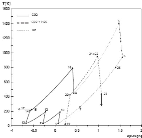
Figure 14. *T - s* diagram of ZEITMOP cycle (Yantovski et al., 2003a).
