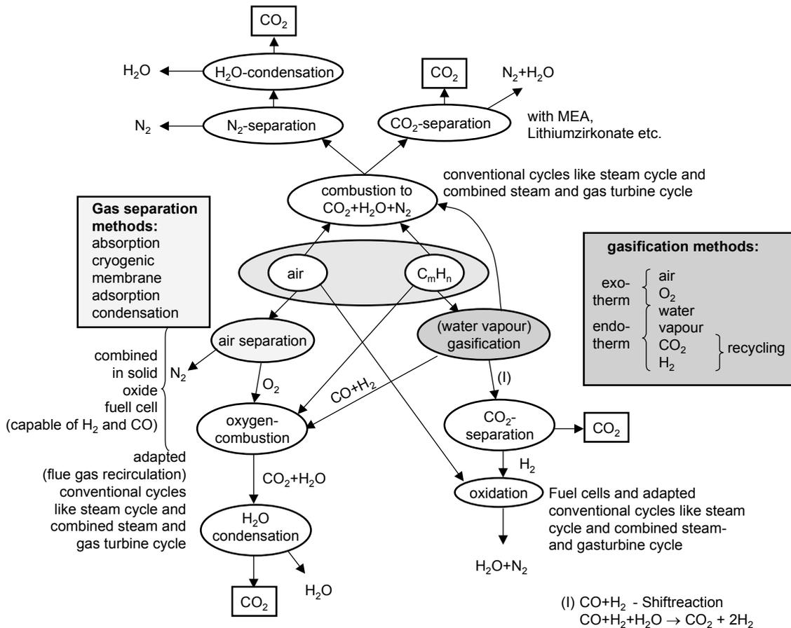
Figure 1. The various methods of carbon capture (Leithner, 2005).
